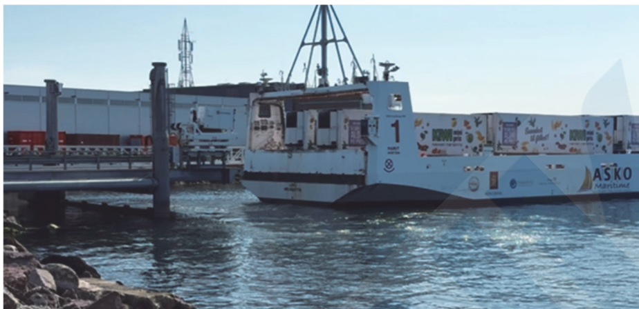
Fig. 1 Automatic berthing of ASKO Marit (going astern)
