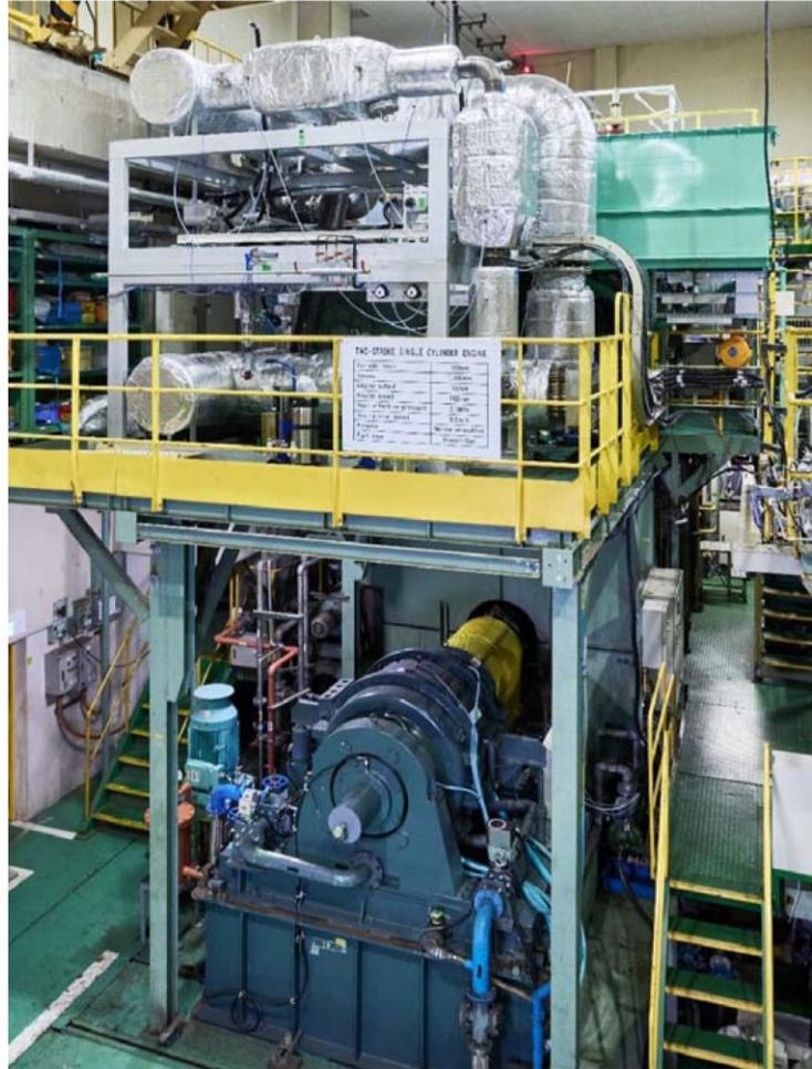
In May 2023, The world's first low-speed 2-stroke engine Ammonia fuel operation has started.
