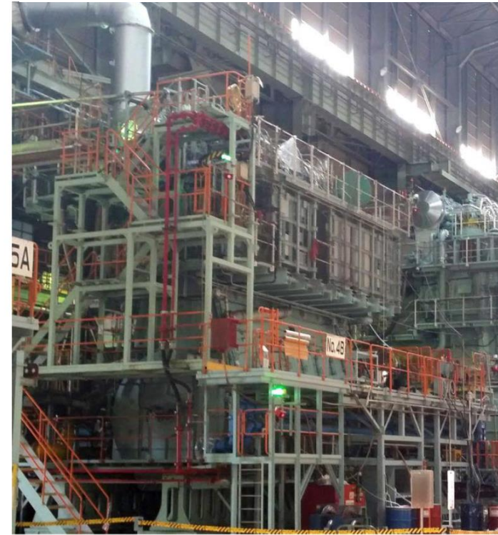
Figure 7 – Picture of the 7S50ME-B9.3-LGI engine on test bed at MES. (CIMAC 2016)
