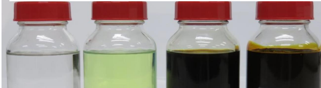
Methanol (Zero sulfur) (Zero aroma) Gas Oil LCO (Low sulfur) (High aroma) CLO
