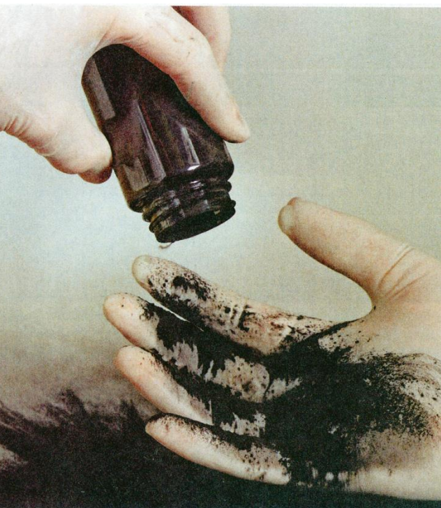
船用軽油からの PM (Soot) (Marine Propulsion, April/May 2010)
