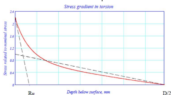
Fig. 3 Torsional SCF in the Crankpin Fillet as a Function of Depth.
