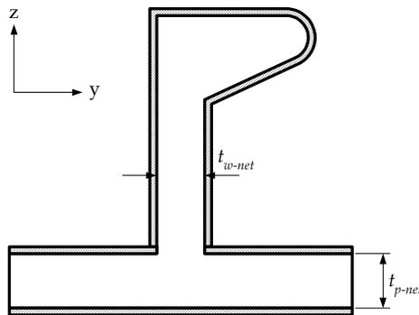
The net cross-sectional area, the moment of inertia about the  $y$ -axis and the associated neutral axis position of the profile is to be determined assuming the corrosion magnitude  $0.5t_{corr}$  deducted from the surface of the profile cross-section, see ~~2.4.1.3~~
