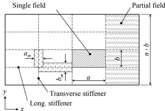
Longitudinal : stiffener in the direction of the length  $a$
