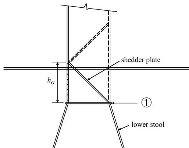
**Fig. 33 Symmetrical gusset/shedder plates (void)**
