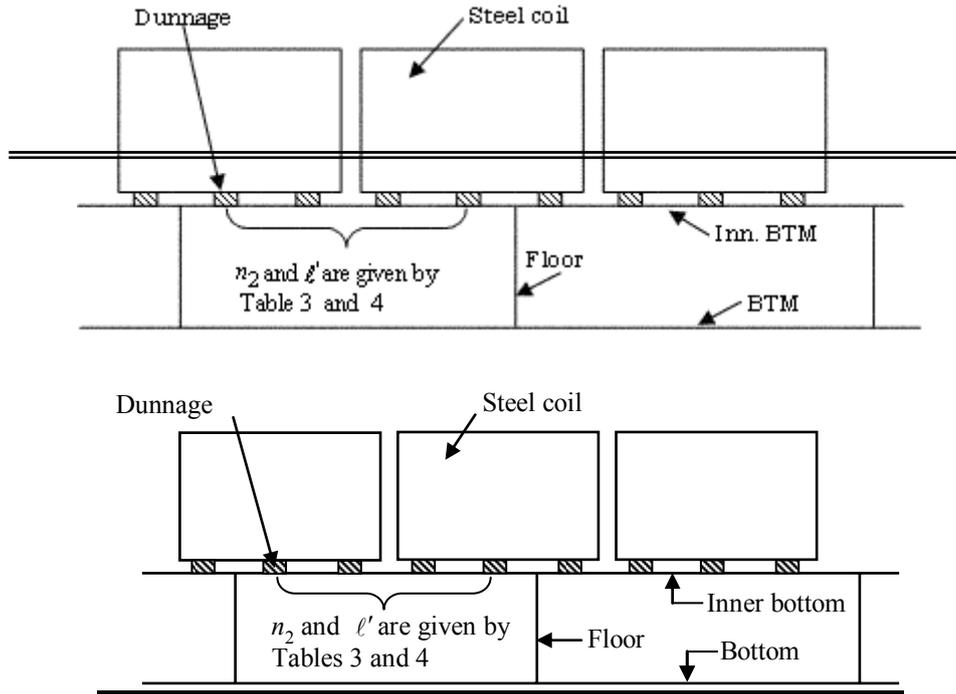
**Fig. 4 Loading condition of steel coils (Example of  $n_2 = 3$ ,  $n_3 = 3$ )**
