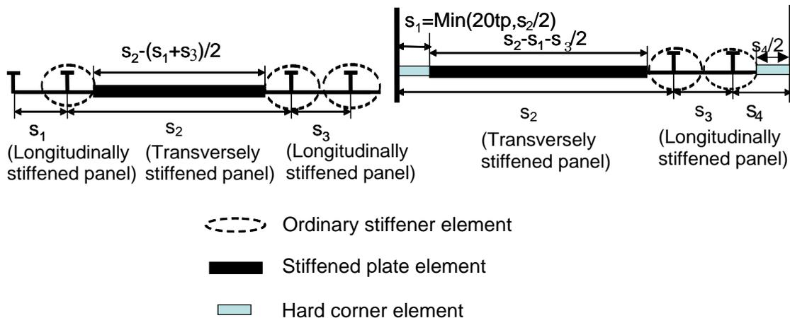
The typical examples of modeling of hull girder section are illustrated in **Figs. 7 and 8.**
