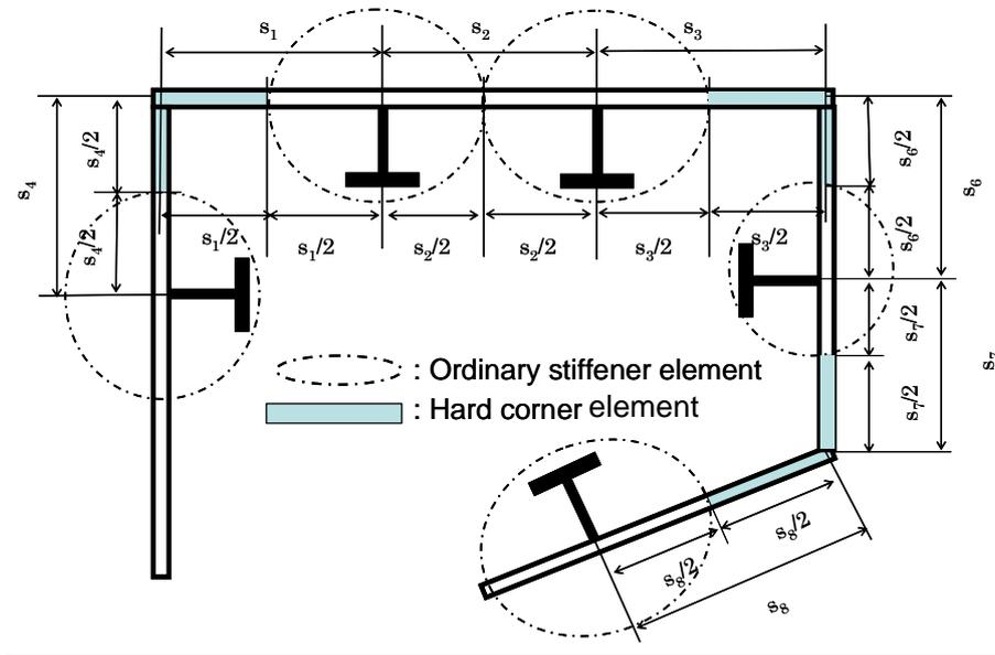
**Fig. 8 Examples of the configuration of stiffened plate elements, ordinary stiffener elements and hard corner elements on a hull section**
