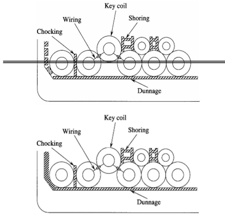
**Fig. 3 Loading condition of steel coils (Example of  $n_2 = 4$ ,  $n_3 = 3$ )**
