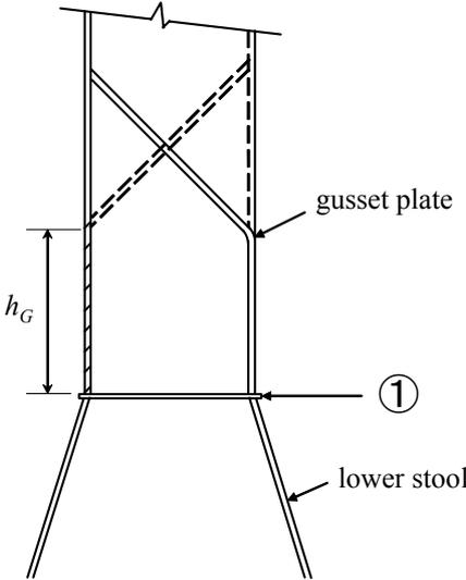
**Fig. 14 Asymmetrical gusset/shedder plates**
