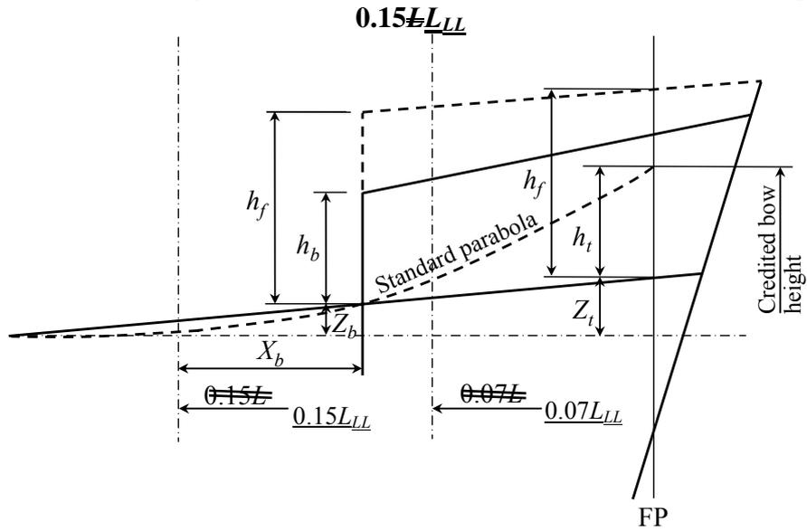
**Fig. 2 Credited bow height where the freeboard deck has sheer extending for less than**
