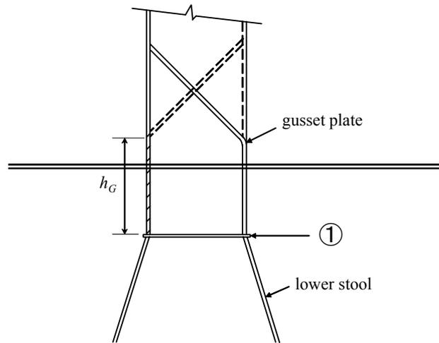
**Fig. 34 Asymmetrical gusset/shedder plates (void)**
