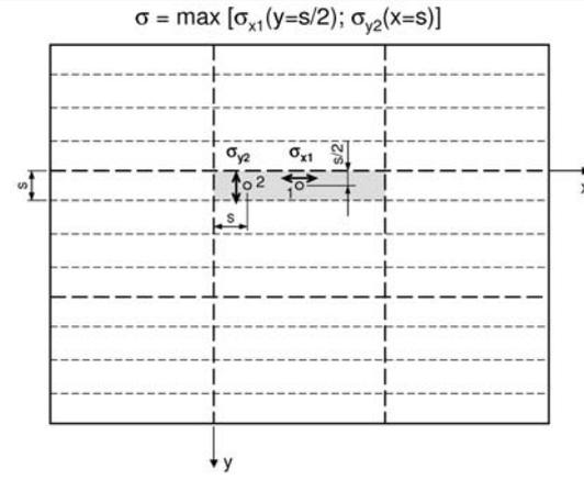
(2) The net thickness of double skin hatch covers and box girders is to be obtained in accordance with 5 below taking into consideration of the permissible stresses specified in 19.2.5-1(1).
