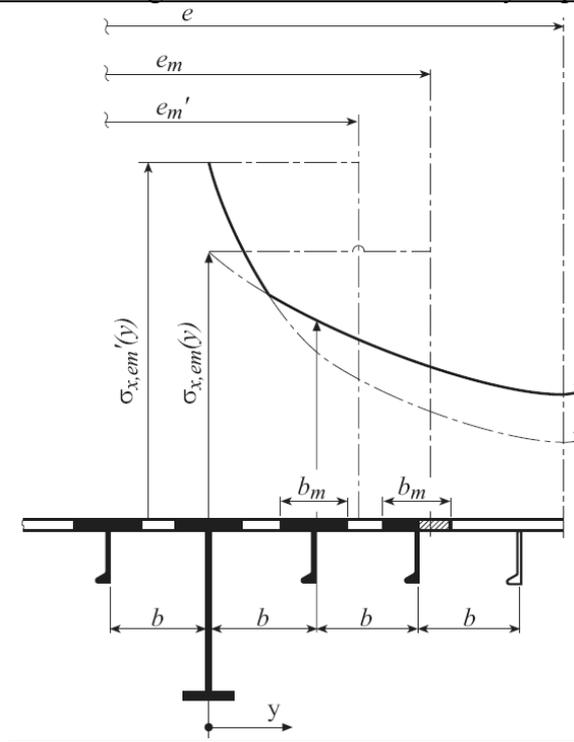
2) Stiffening perpendicular to the webs of primary supporting members (see Fig. CS19.6). For  $a < e_m$ ,  $a$  and  $b$  have to be exchanged.
