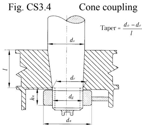
The taper length  $l$  of rudder stocks fitted into the rudder plate and secured by the slugging nut is generally not to be less than 1.5 times the rudder stock diameter  $d_o$  at the top of the rudder. In this case, for couplings between stock and rudder, a key is to be provided. The scantling of the key is to be to the discretion of the Society.
