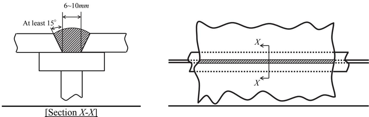
(b) Continuous slot welding
