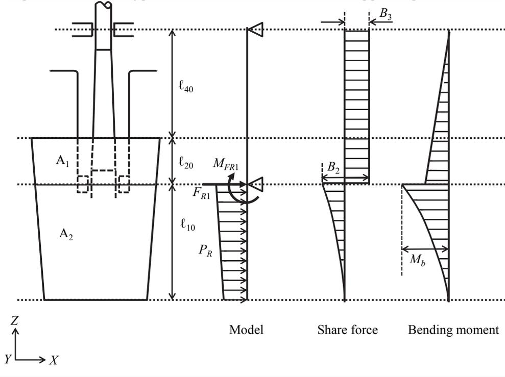
Fig. C3.4.1-7 Type D Rudder with 2-conjugate elastic supports
