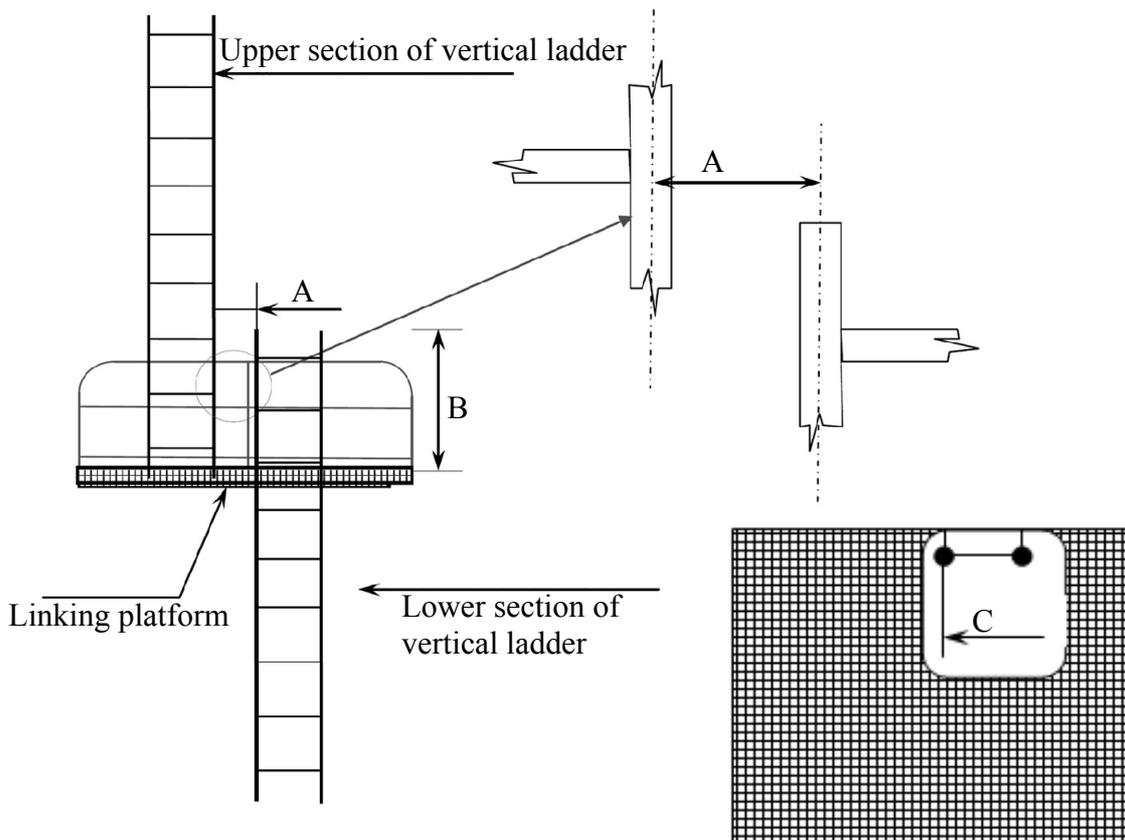
Fig. C35.2.3-2 Vertical ladder - side mount
