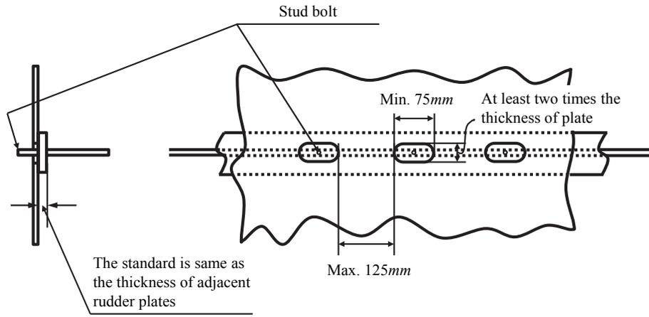
Note: The standard leg length of slot welding is  $F_{L2}$ .
