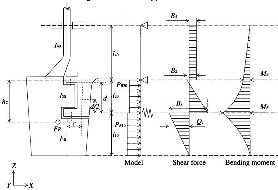
Fig. C3.4.1-6 Type C Rudder with rudder trunk supporting rudder stock
