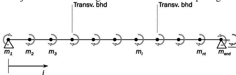
$m_{hi}$  can be substituted to  $m_{vi}$  in this figure and  $m_i$  is the positive bending moment in FE coordinate system.
