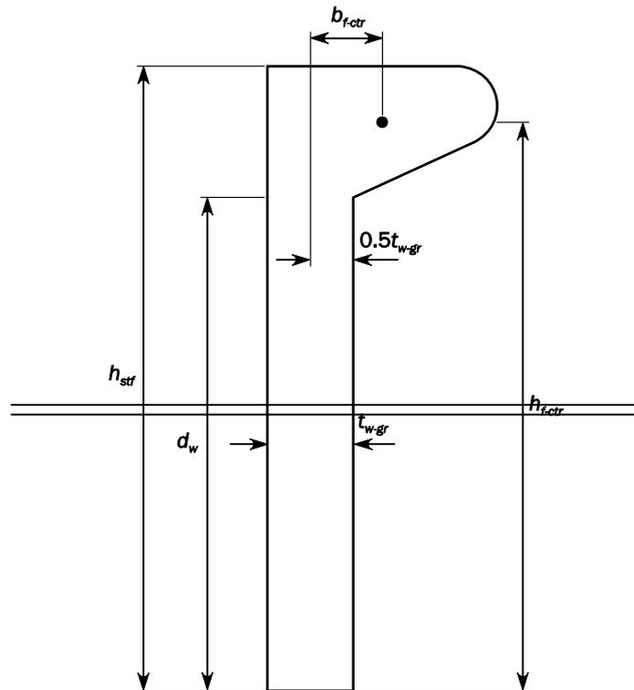
~~Fig. 1615~~ Effective Shear Area in way of Web Openings
