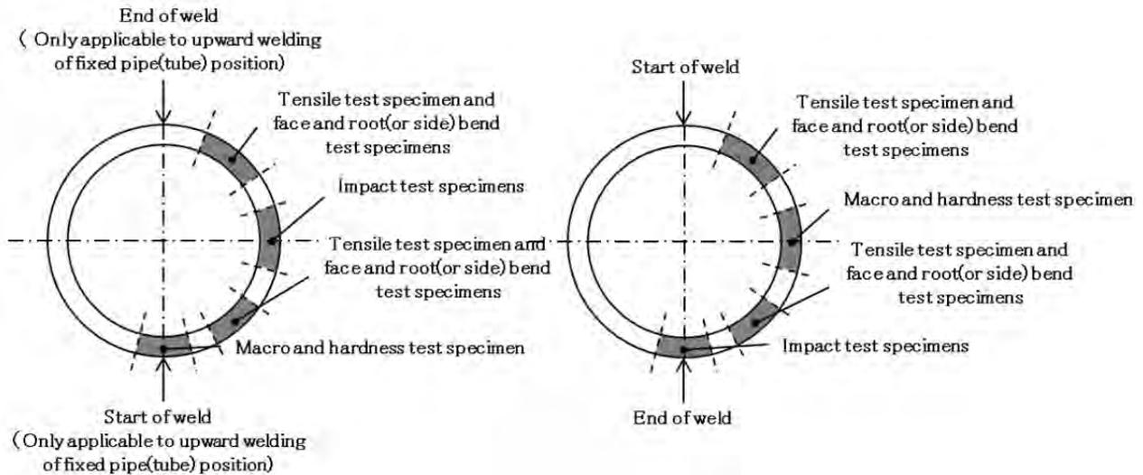
(B) Test Assembly for pipes (or tubes)
