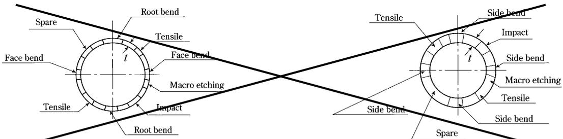
(B) Test Assembly for Pipes up to 20 mm in Thickness
