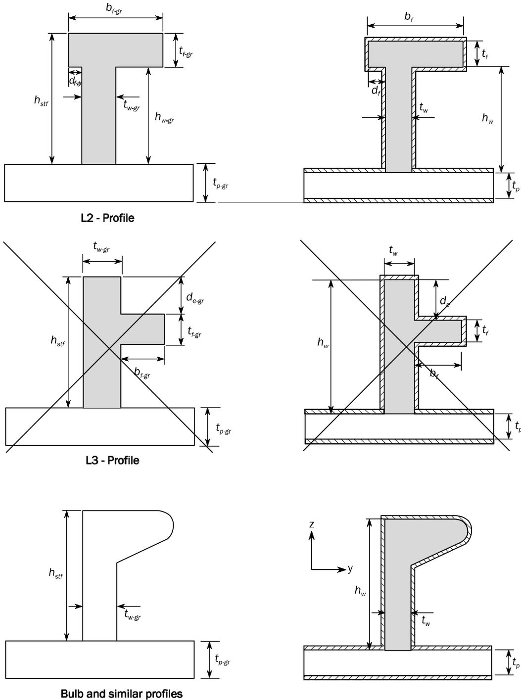
The net cross-sectional area, the moment of inertia about the  $y$ -axis and the associated neutral axis position are to be determined applying a corrosion magnitude of  $0.5 t_c$  deducted from the surface of the profile cross-section.
