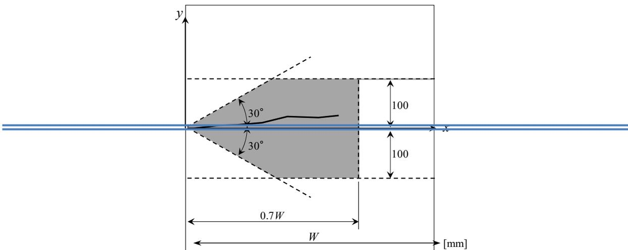
~~(2) The arrest crack length,  $a$ , is to satisfy the following (a) to (c) formulae. However, if the strain at the pin position and the crack length at the pin position have been dynamically measured and the value of the strain at the time of arrest is 90% or more of the static strain immediately before crack initiation, the application of formula (c) is not necessarily needed.~~
