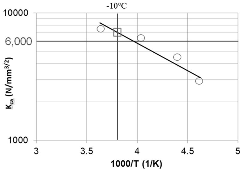
Fig. 92 Evaluation Example of Temperature Corresponding to Required  $K_{ca}$
