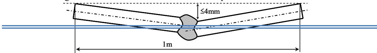
3 — The accuracy of in-plane and out-of-plane loading axes are shown in Fig. 5. The accuracy of the in-plane loading axis is to be 0.5% or less of the distance between the pins, and the accuracy of the out-of-plane loading is to be 0.4% or less of the distance between the pins. Stress in a loaded test specimen is to be uniform.
