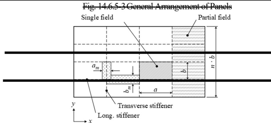
Longitudinal : stiffener in the direction of the length  $a$
