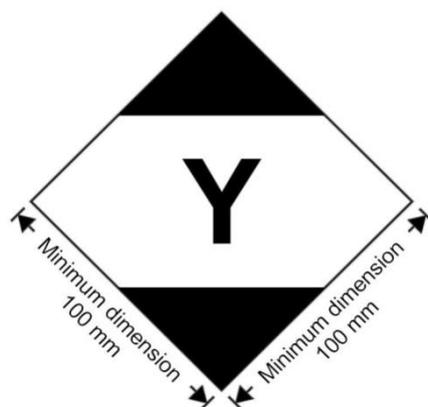
Marking for packages containing limited quantities conforming to Part 3, Chapter 4 of the ICAO Technical Instructions for the Safe Transport of Dangerous Goods by Air.
