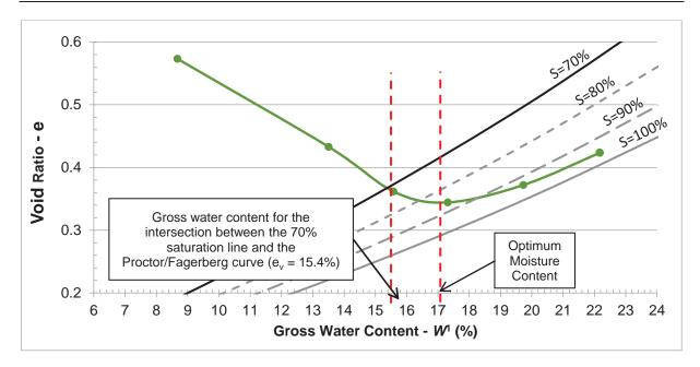
Figure 1.5.10 Example of a measured compaction curve for void ratio versus gross water content with the 70%, 80%, 90% and 100% degree of saturation lines plotted
