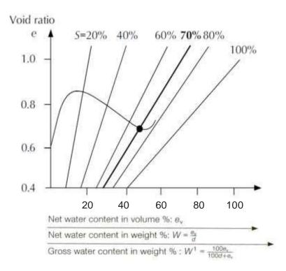
Figure 1.5.9 Typical compaction curve
