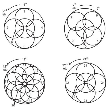
Figure 1.5.6 Recommended compaction patterns
