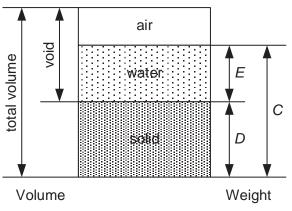
Figure 1.5.5 Illustration of key variables
