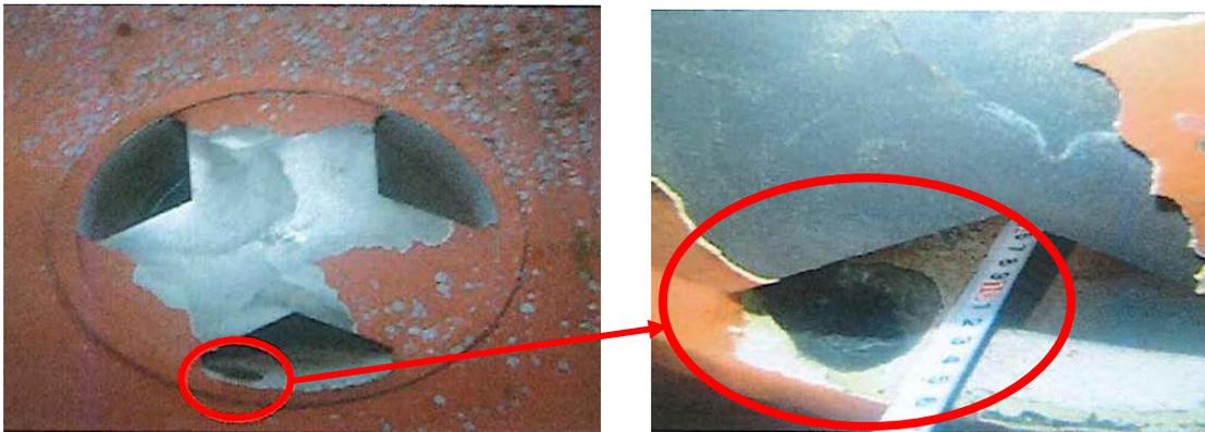
Picture 2 Corrosion on/around welded parts between distance pieces and bluff bodies
