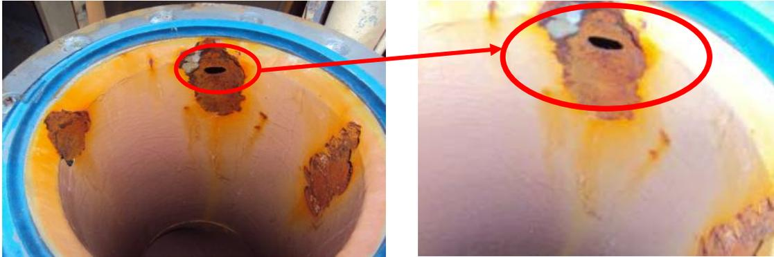
Picture 1 Damage on/around welded parts between distance pieces and flanges
