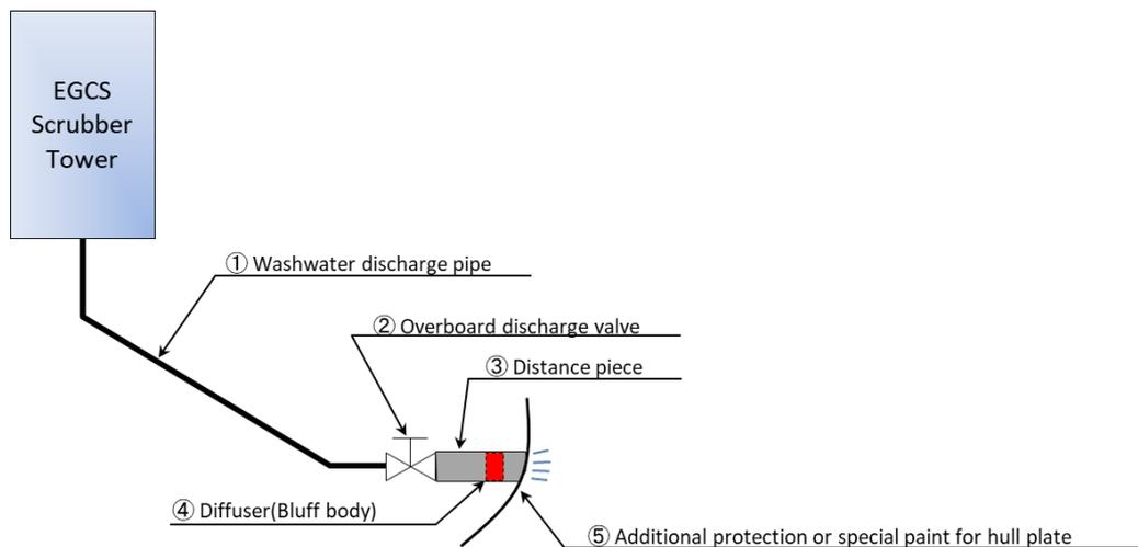
Figure 1 SOx scrubber discharge water line
