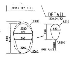
3 If a vertical opening is at a height of more than 600 mm steps then handgrips should be provided. In such arrangements it should be demonstrated that an injured person can be easily evacuated.
