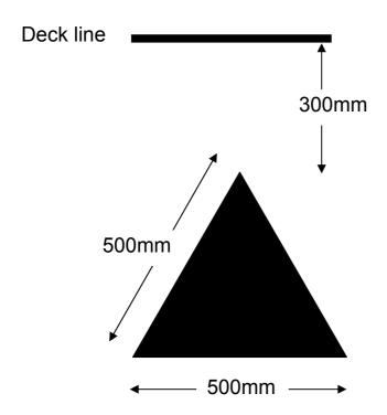
The permanent marking, of a solid equilateral triangle is to be made on the side shell at midships, port and starboard, by punching, weld beads or cut out of a thin plate welded.
