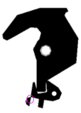
Picture 2.2 Insufficient holding
