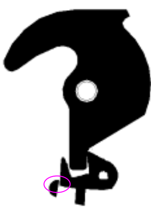
Picture 2.1 Insufficient holding
