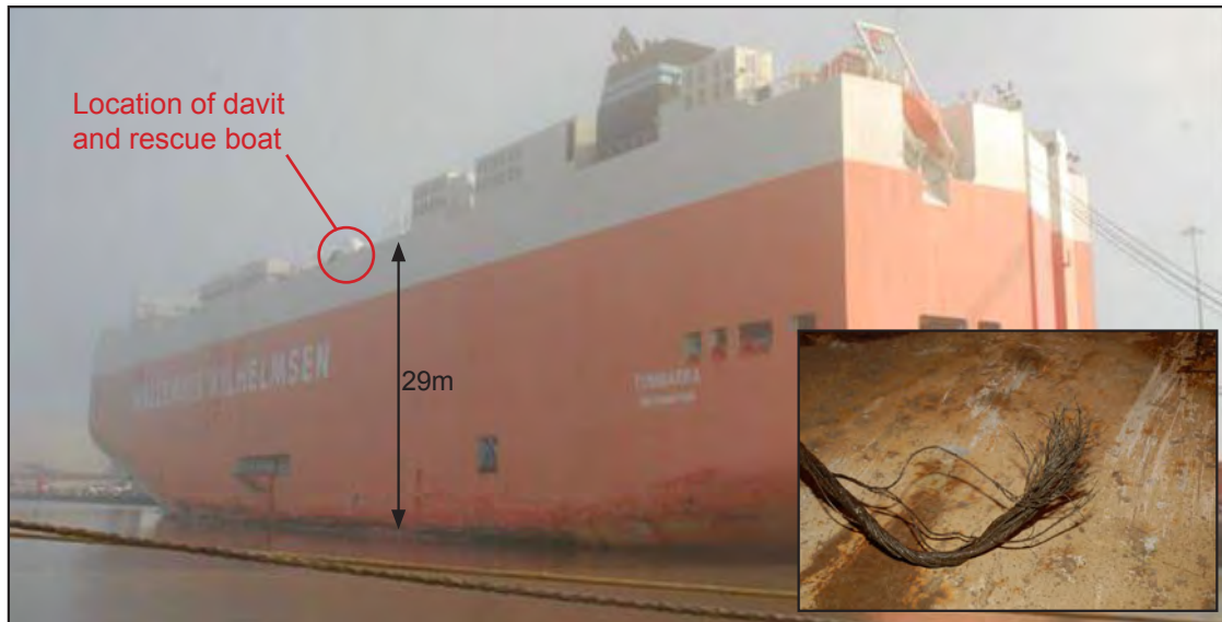
Vessel and parted fall wire
