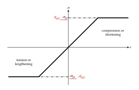
b) Typical stress strain curve  $\sigma$ - $\varepsilon$  for elasto-plastic failure of a stiffener
